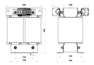
• Equipped with two temperature sensors PT100, thanks to these sensors, the transformers work better with HAKEL ISOLGUARD insulation monitoring devices and provide the best possible basis for measuring the insulation status and transformer heating.
